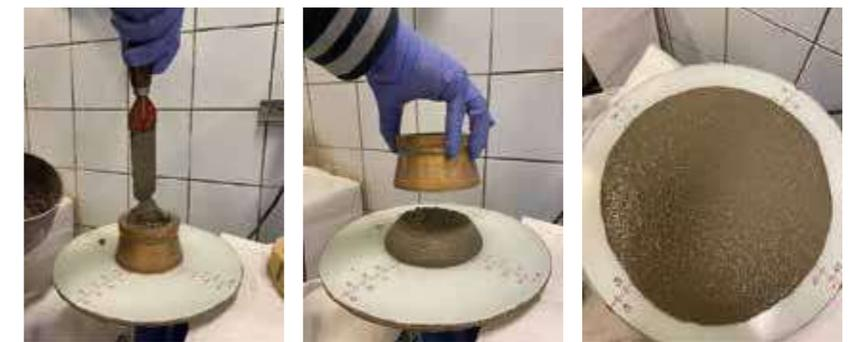
2. Flow test used to assess the workability of cements.
