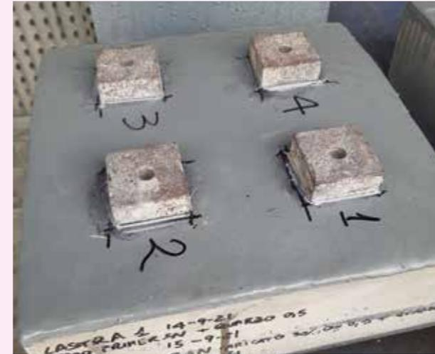
3. Pull-off test to evaluate adhesion to a cementitious substrate.
