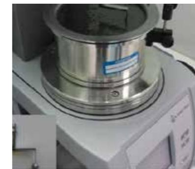
8. Rheometer equipped with a ball measuring system.
