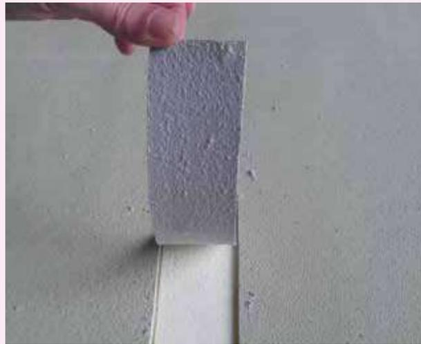
1. Peel-strength test of polyurea.
